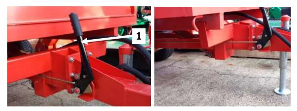
Align the tractor's rear drawbar to the pin hitch (2) on the trailer. Then raise or lower the trailer hitch using the stand (3). The handle can be used to wind the trailer up so the trailer and tractor hitching points are aligned. Then insert the tractor pin through the drawbar and trailer hitch to secure in place.
