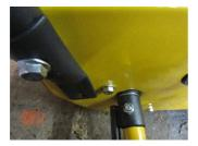
Step 1. Remove the 2x12mm bolts to allow the handle to drop into position.
