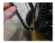
Step 4. Attach the gear lever using 2x10mm bolts
