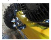
Step 3. Remove the 2x10mm bolts which are for the gear lever
